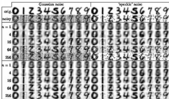
Figure : Denoising of the USPS dataset. Orig. dataset, followed by noisy version. The next five rows : reconstruction for linear PCA using different k values. The last five rows : reconstruction using the approximate preimage approach with kernel PCA.
